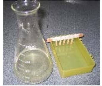
4. Once the solution is cool enough to pour, add just enough into the box so that ~0.5 cm of the comb teeth are submerged. Adjust the comb by sliding it so that it is ~1.5 cm from the top of the box. Thinner gels will yield better separations.
