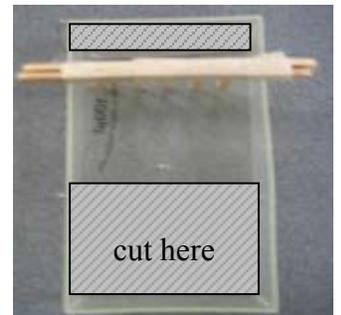
6. Bend each piece of stainless steel wire to run along the width of the box and hook over the side. Place one on either side of the gel. Use tape to secure them to the box if you need to. These will be the positive and negative electrodes.
