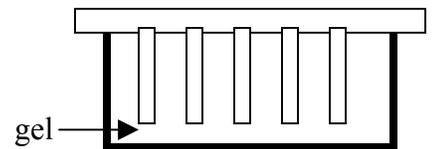
5. The actual gel only needs to be half the size of the box. In addition, you need to make space to place the electrodes. Once the gel sets (~5-10 min), use a knife to cut off the bottom half of the gel. Also, without disturbing the comb, cut out a thin strip from the top of the gel to make room for a wire electrode. Your gel should now be around 6 cm long and 8 cm wide (still the full width of your box). You can recycle the pieces of gel that you cut out by reheating them in the microwave.
